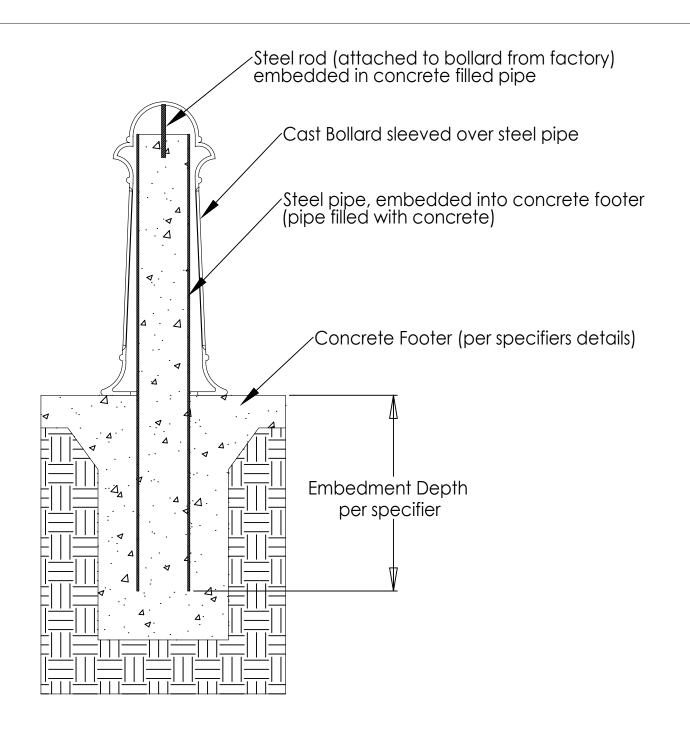
Cast Bollard over Steel Pipe Typical
